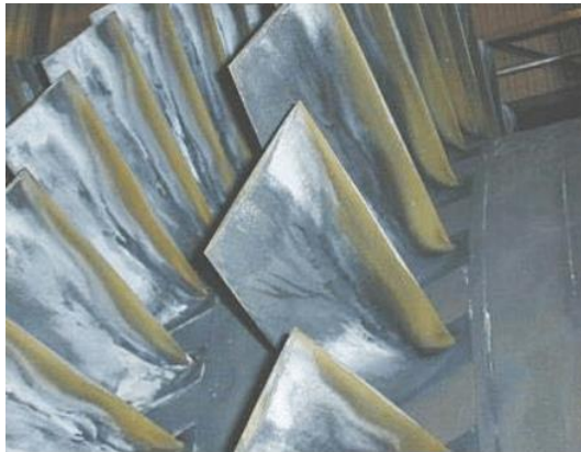
FIGURE 8. - Heavy hydrated salts fouling in a typical axial compressor Surface roughness
