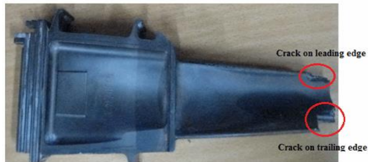
FIGURE 9. - Failed first stage high pressure gas turbine blade collected from site
