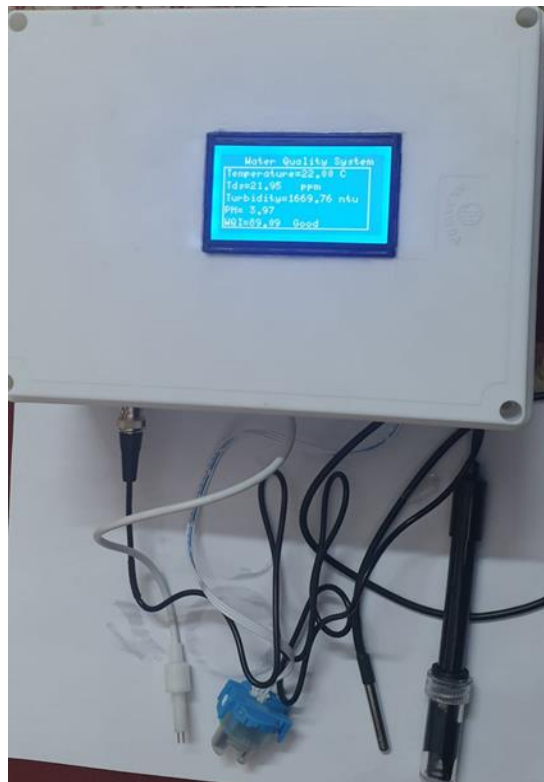
FIGURE 1. - WQMS hardware components
