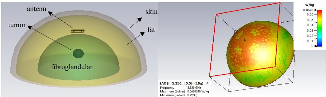
**FIGURE 3. breast model with one antenna inside the fat layer and SAR major**
