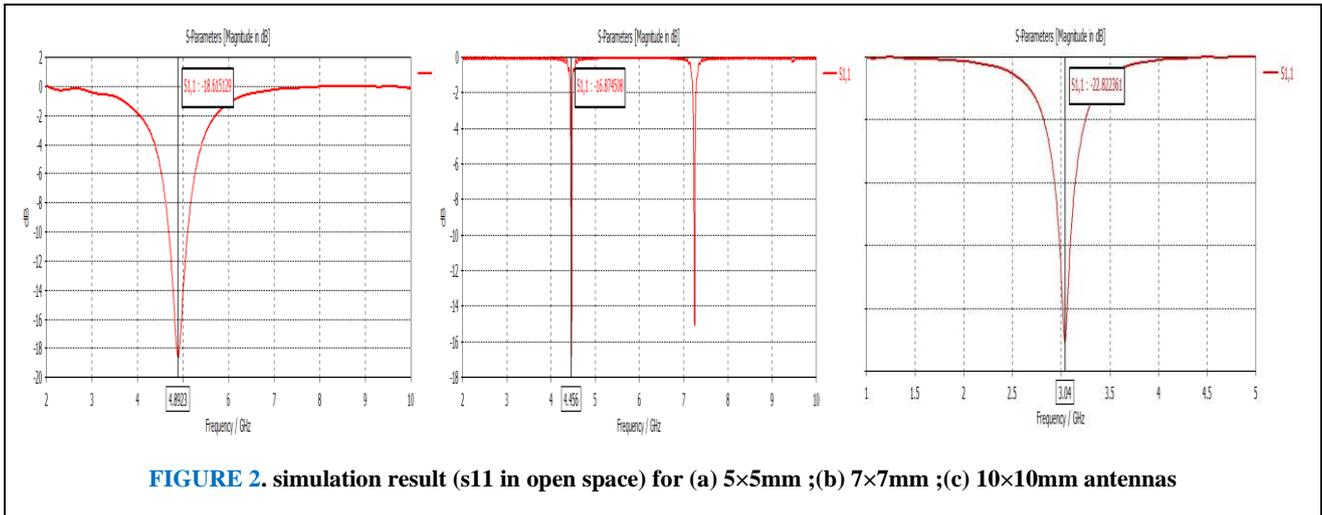
FIGURE 2. simulation result (s11 in open space) for (a) 5×5mm ;(b) 7×7mm ;(c) 10×10mm antennas
