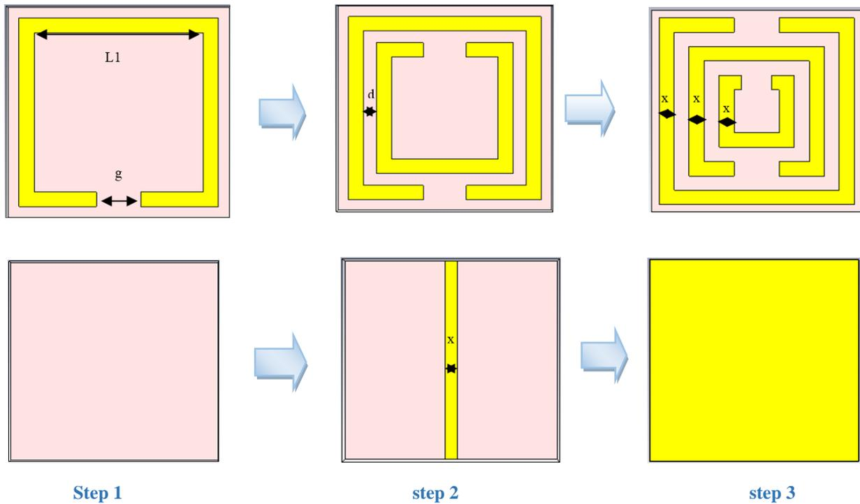
**FIGURE 1. steps for antennas front and back design step 2 for antenna size (5,10)mm and step3 for (7)mm antenna size**
