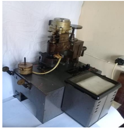
Figure 1 General view of the four-ball friction machine (KT-2)
