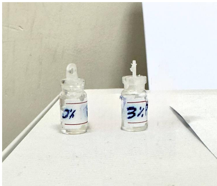
FIGURE 2. - Fresh glass cups containing (0%, 3%, SP essential oil modified adhesive discs) rinsed in water for oil leaching tests
