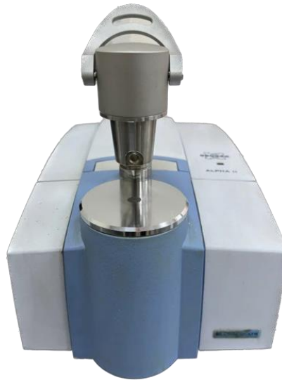
FIGURE 3. - Fourier-transform infrared spectrophotometer (Alpha II, Platinum, Bruker Optic GmbH, Ettlingen, Germany)
