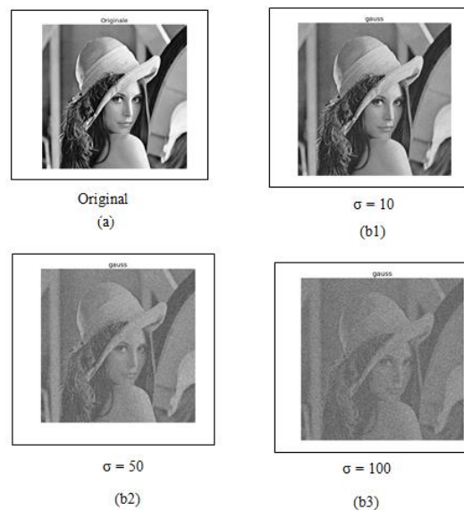
FIGURE 6. - Difference between the original picture (a) and the three-level Gaussian noise image (b1, b2, b3) ( \sigma=10 , \sigma=50 , \sigma=100 )
