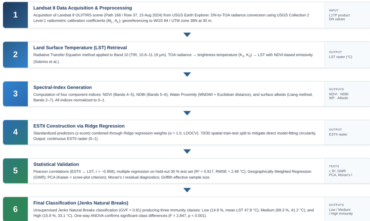
FIGURE 2 Schematic workflow of the ESTII methodology, summarising the major stages: (1) Landsat 8 data acquisition and preprocessing; (2) LST retrieval from Band 10; (3) spectral-index generation (NDVI, NDBI, WP, Albedo); (4) ESTII construction via Ridge regression; (5) statistical validation (Pearson, 70/30 internal split, GWR, PCA, Moran's I); and (6) final Jenks Natural Breaks classification into Low / Medium / High immunity classes
