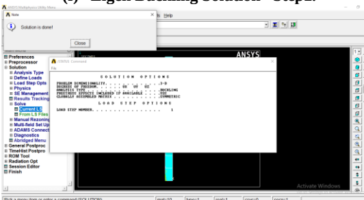
(h) Eigen Buckling Solution– Step4.
